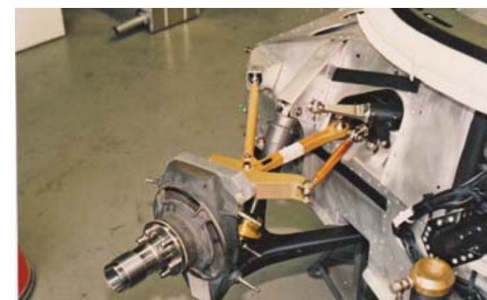
LH Front corner – note slots in upright for airflow to disc and Titanium hub and wheel drive pegs
