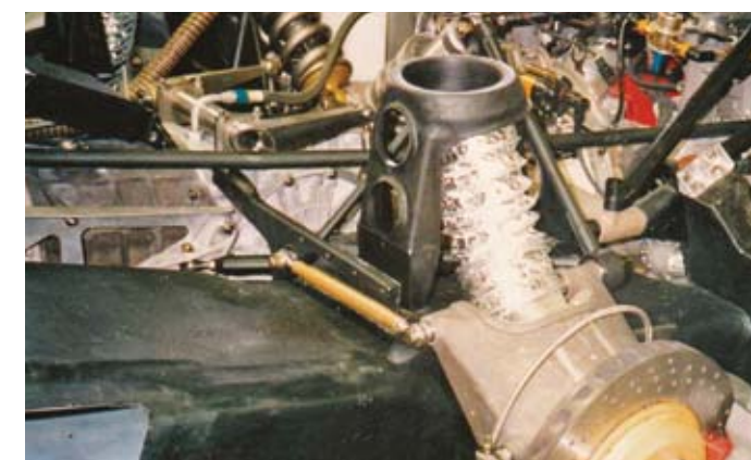
Detail of RH rear upright and brake cooling
