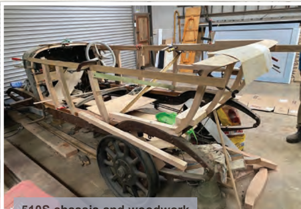
510S chassis and woodwork
